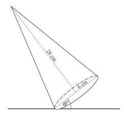
A uniform solid cone has vertical height 28 cm and base radius 6 cm. The cone is held with a point of the circumference of its base in contact with a horizontal table, and with the base making an angle of  $\theta^{\circ}$  with the horizontal (see diagram). When the cone is released, it moves towards the equilibrium position in which its base is in contact with the table. Show that  $\theta < 40.6$ , correct to 1 decimal place. [3]
